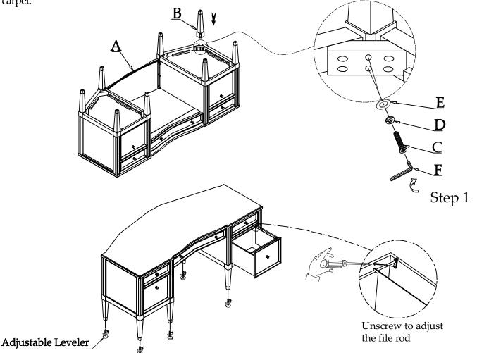
The File Drawer can be set up to use either Letter or Legal size hanging file folders using the File Rods installed in the file drawers.
